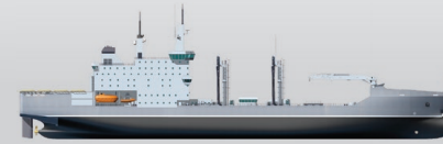
Resolve-Class Auxiliary Oiler Replenishment Ship Displacement: 26,000 tonnes
