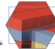
CONTAINERISED STORAGE AREA A protected, environment-controlled area for the storage of containerised stores, supplies and ammunition serviced by cargo elevators for packing / unpacking while at sea
